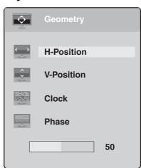
**H-Position**—Moves the monitor image left and right. **V-Position**—Moves the monitor image up and down.
